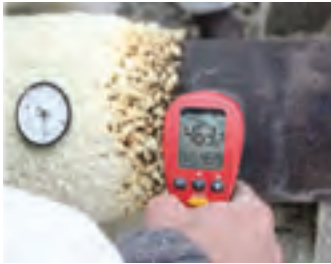
Before HPC® Coating application 865.4°F (463°C)
