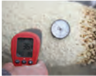
After HPC® Coating application 96.8°F (36°C)
