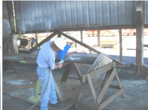
A piece of 8 " Schedule 40 pipe was preheated with a Tiger Torch.
