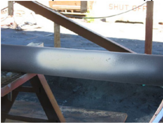
A temperature reduction from 350C on the bare pipe to 170C after the initial primer coat @ 50 mils (1.2mm) DFT was applied.
