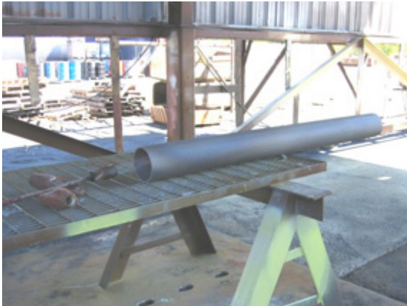
A piece of 8 " Schedule 40 pipe was preheated with a Tiger Torch.
