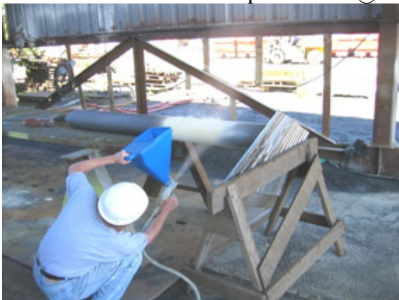
A temperature reduction from 370C on the bare pipe to 90C after the second primer coat @ 50 mils (1.2mm) DFT was applied. ( Video )
