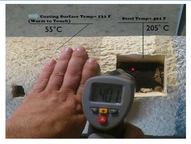
Inspection windows can be cut out of the coating film over weld joints for repeat non destructive inspection.
