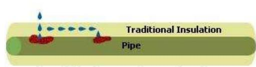
Rockwool, fiberglass, or other traditional types of insulation promote corrosion, and also act as a carrier and spread the corrosion to other areas of the pipeline
