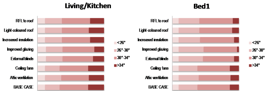
Figure 1.2: Proportion of time at temperatures during 4-day heat wave
