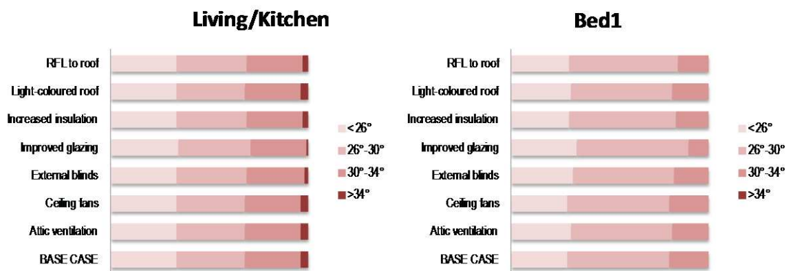
Fig 1.4: Proportion of time at temperatures during 4-day heat wave
