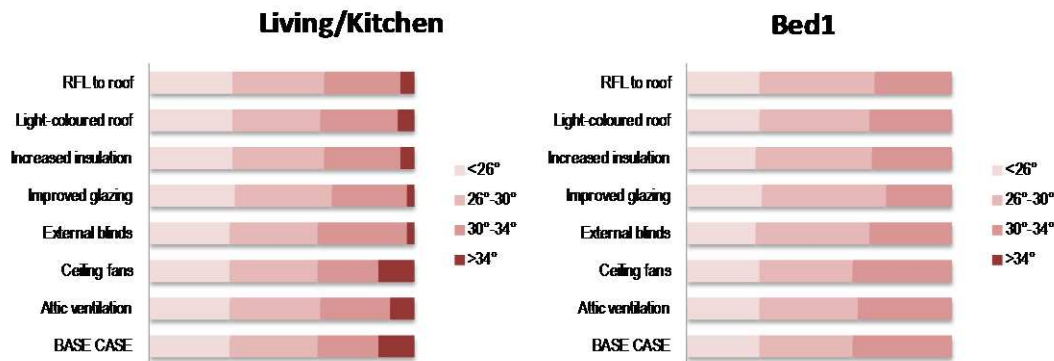
Figure 1.3: Proportion of time at temperatures during 4-day heat wave
